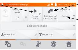
Switching Unidirectional/Bidirectional measurement.
