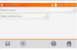
Enter and save the material and  $\alpha$  coefficient, using the same method as described in section 2.2.4.
