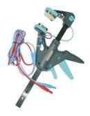
Kelvin clamp with a 2.6 m double-wire cable (for I ≤ 10 A)
