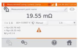
In addition to the resistance, the meter also displays the value of current measured with clamps.
