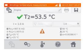
R<sub>T1</sub> - resistance of the cold winding
