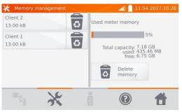
This option allows you to read the % of the used memory and to clear it: after clicking **Delete memory** all clients are deleted with their objects and measurement results. By pressing button oldow located next to each customer, you can also delete individual customers.
