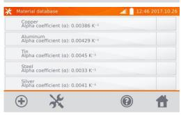
The meter has 5 defaults materials saved in the memory, together with the thermal resistance coefficients of: copper, aluminium, tin, steel and silver. Use button to add a new material.
