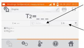
The method of supplying the measuring current is non-adjustable and set on Auto mode - the measuring current is limited to a value not exceeding the set value.
